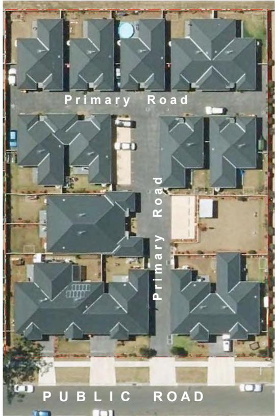
Fig 4-2: (above) Multi-dwelling Housing 'Mews'. As-built impact accommodating vehicles within a site
